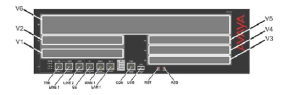
The following tables describe the functions of the fixed ports and buttons on the G350 front panel.
